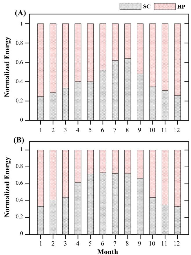
Fig. 18. Comparison of monthly energy requirements of dual-tank solar combisystems in (A) Taipei and (B) Kaohsiung.
