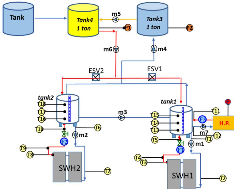
Fig. 2. Schematic of the solar combisystem equipped with sensors.
