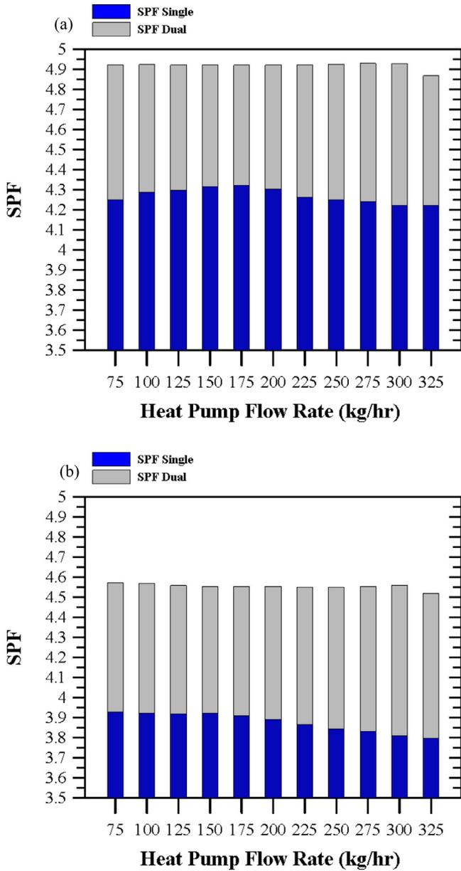
Fig. 19. Seasonal performance factors for systems of various heat pump flow rates with different system layouts in (a) Kaohsiung and (b) Taipei.
