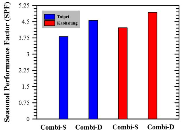
Fig. 21. Seasonal performance factor differences between single-tank and dual-tank combisystems in Taipei and Kaohsiung.
