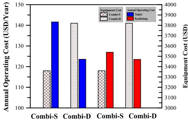
Fig. 22. Annual operating cost and equipment cost differences between single-tank and dual-tank combisystems in Taipei and Kaohsiung.
