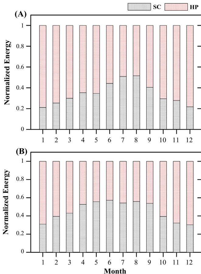
Fig. 17. Comparison of monthly energy requirements of single-tank solar combisystems in (A) Taipei and (B) Kaohsiung.
