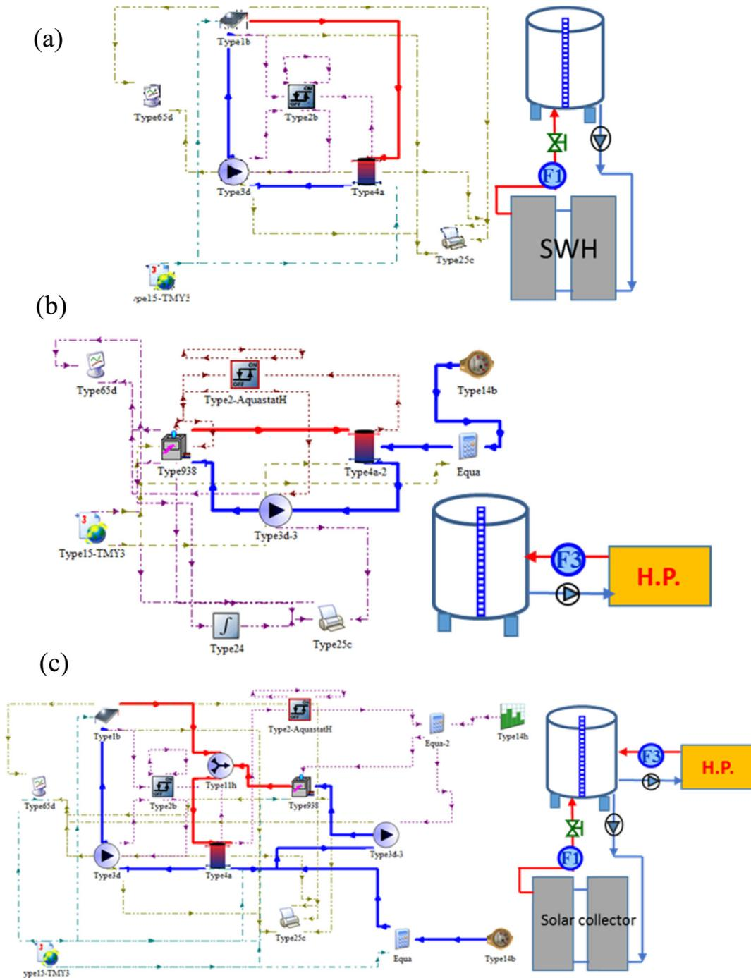
Fig. 3. Solar domestic hot water system (a) SWH system (b) HP system (c) Single tank combisystem.
