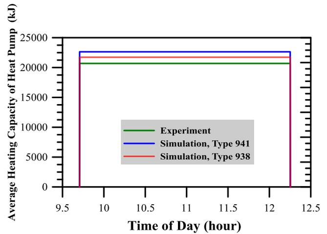
Fig. 6. Average heating capacity of heat pump according to numerical simulation and experimental demonstration.
