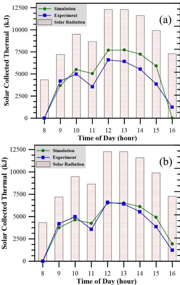
Fig. 5. Solar collected thermal energy values from numerical simulation and experimental demonstration (a) default parameter settings, (b) adjusted parameter settings.
