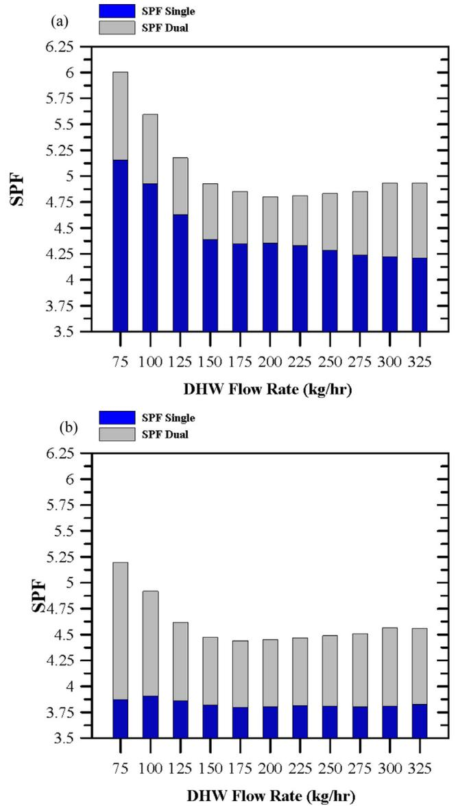
Fig. 20. Seasonal performance factors for systems of various domestic hot water flow rates with different system layouts in (a) Kaohsiung and (b) Taipei.
