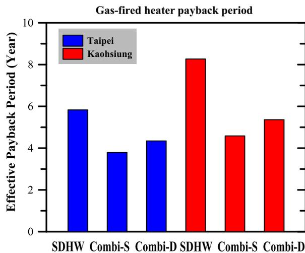
Fig. 23. Payback periods (relative to gas heaters) for three different types of domestic hot water systems in Taipei and Kaohsiung.
