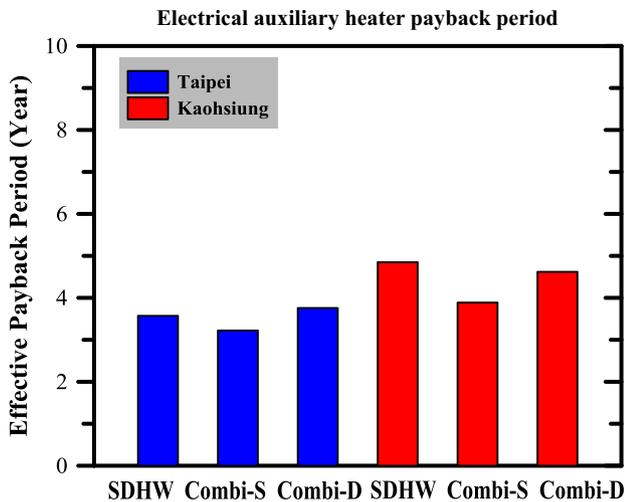
Fig. 24. Payback periods (relative to electric heaters) for three different types of domestic hot water systems in Taipei and Kaohsiung.
