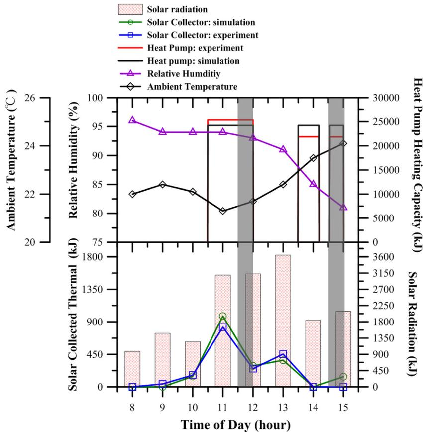
Fig. 7. Heat transfer of solar collector and heat pump domestic hot water system.
