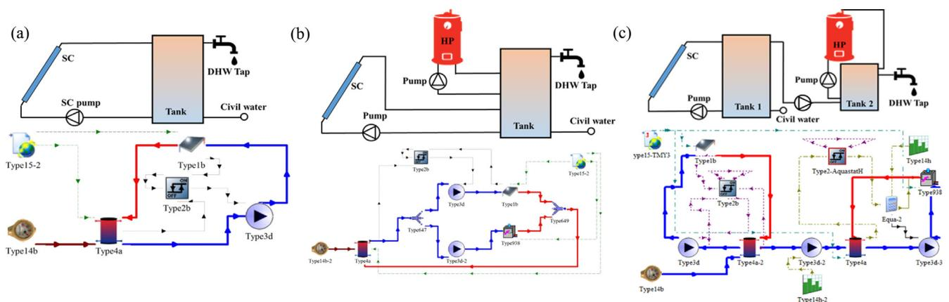
Fig. 4. Layout of SDHW systems (a) SWH system (b) Single tank combisystem (c) Dual tank combisystem.
