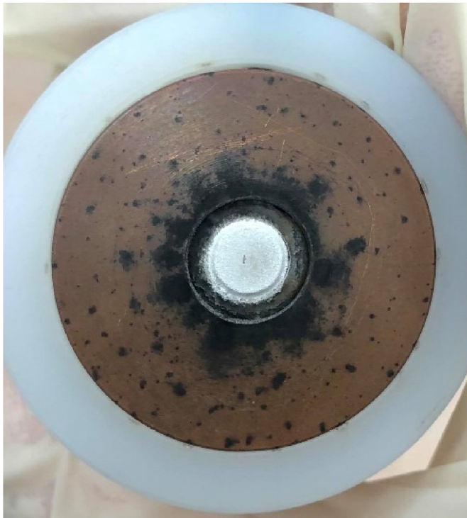
Fig. 21. VAT surface image was taken after life test.
