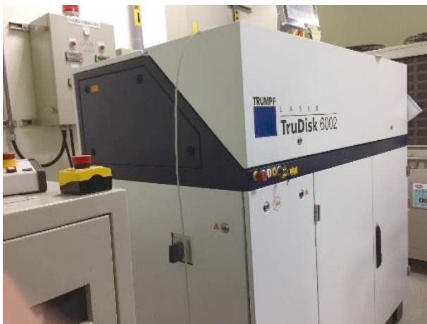
Fig. 3 The TRUMPF TruDisk 6002 laser used for the current laser-cladding experiment.
